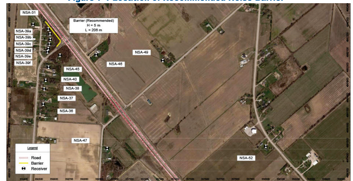
Figure 7-1 Location of Recommended Noise Barrier
